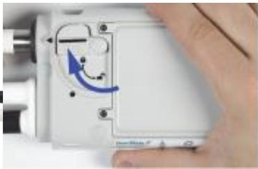
1. To insert the driveline, slide the safety tab back to unlock and expose the red button
